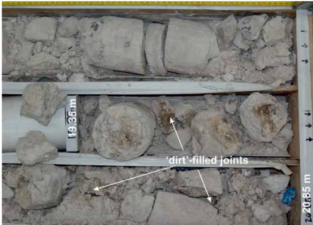
Figure C5a9 Dirt-filled 'open' joints, CIRIA grade C.
