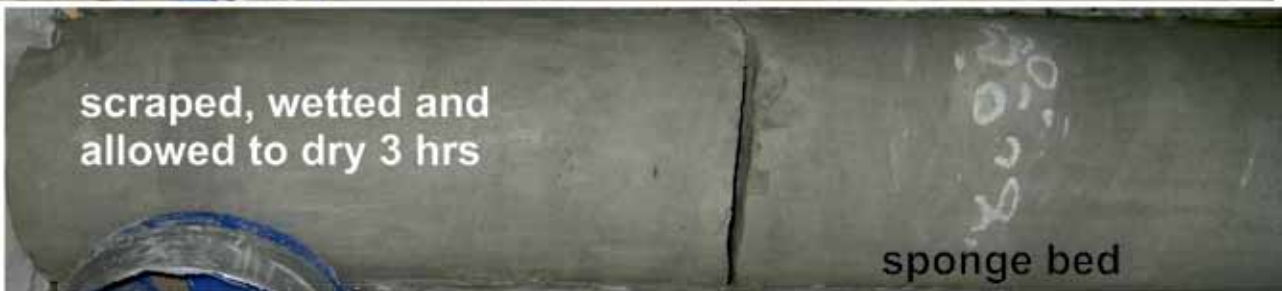
Figure C5d1 West Melbury Marly Chalk Formation core from Offham B borehole, Lewes, Sussex illustrating the enhancement of lithological detail as the core is scraped clean, washed with a squeeze bottle and allowed to dry.
