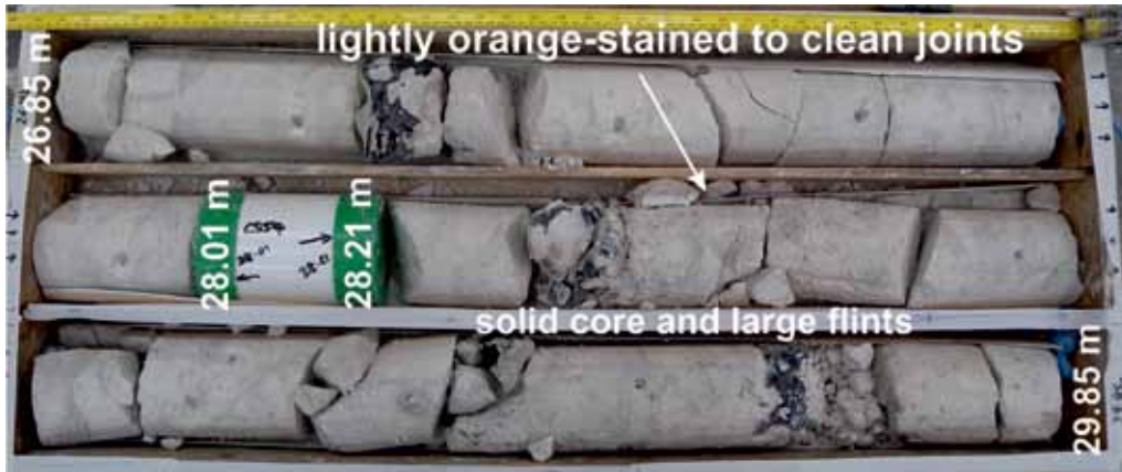
Figure C5a15 Continuously solid core (mostly drilling-induced fractures) with large flints and clean closed joints, CIRIA grade A.
