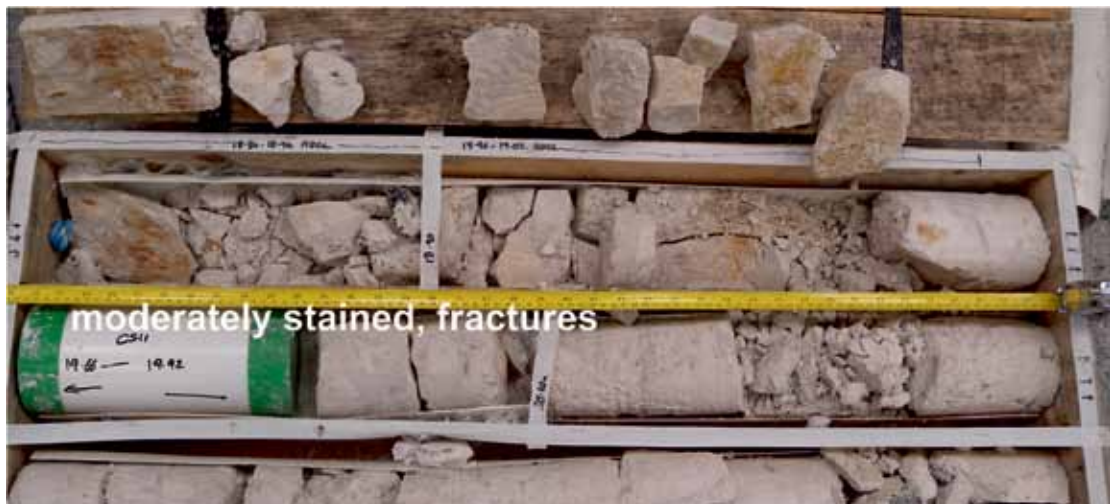
Figure C5b4 Next box fractures are open <3 mm, moderately stained, hence CIRIA grade B.
