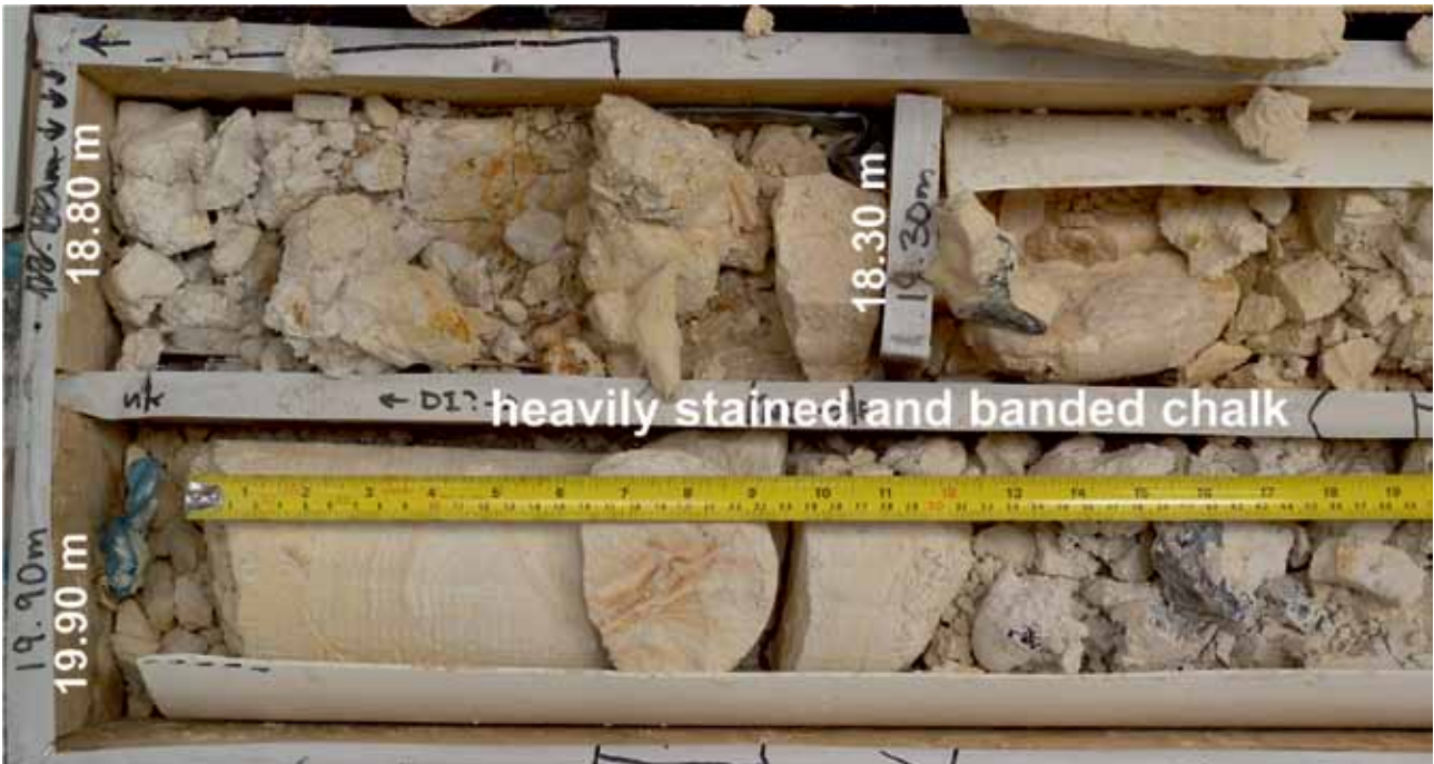
Figure C5c5 Box 4, heavily stained and Liesegang banded chalk and disintegrated core where flints are present. Some solid core with stained fractures, CIRIA grade B, locally C.
