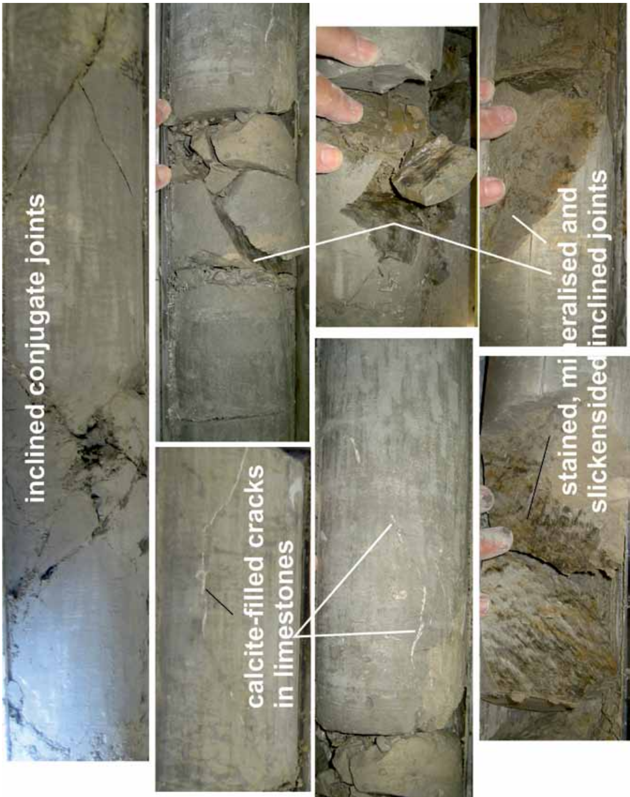
Figure C5d2 Shears, joints and calcite-filled cracks in the West Melbury Marly Chalk Formation, Offham B borehole, Lewes Sussex.
