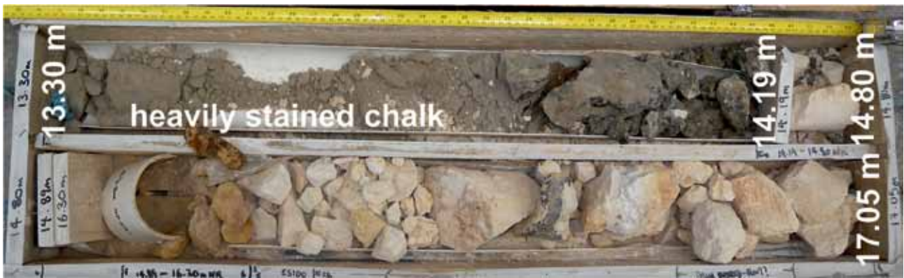
Figure C5c1 Box 2, heavily stained chalk and core loss. Despite the poor core recovery, a ‘blocky’ structure is retained and, combined with the staining, suggests CIRIA grade C.
