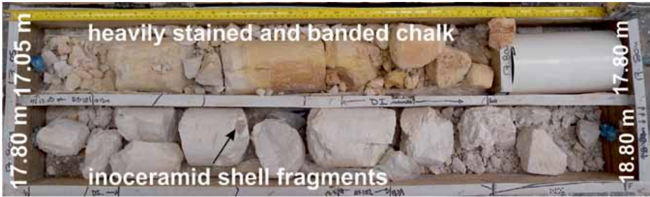
Figure C5c3 Box 3, heavily stained chalk with drilling-induced fractures and fragmentation and some solid core indicating structured chalk, CIRIA grade B.
