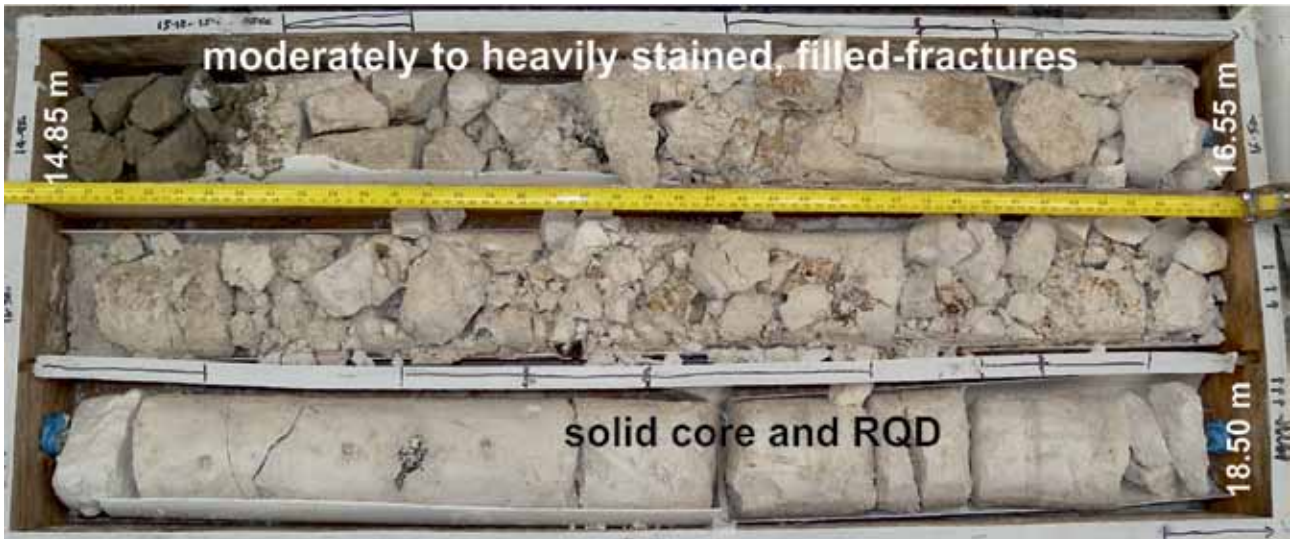
Figure C5b1 Fractures in first 2 m below Thanet contact are open >3 mm, stained and filled, hence CIRIA grade C.
