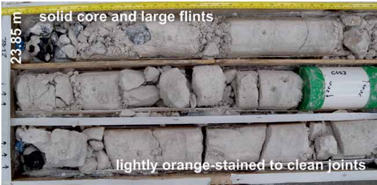
Figure C5a13 Continuously solid core (mostly drilling-induced fractures) with large flints and clean, closed joints, CIRIA grade A.
