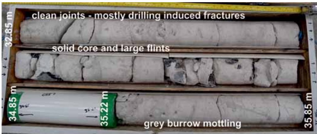
Figure C5a16 Continuously solid core (mostly drilling-induced fractures) with large flints and clean closed joints, CIRIA grade A.
