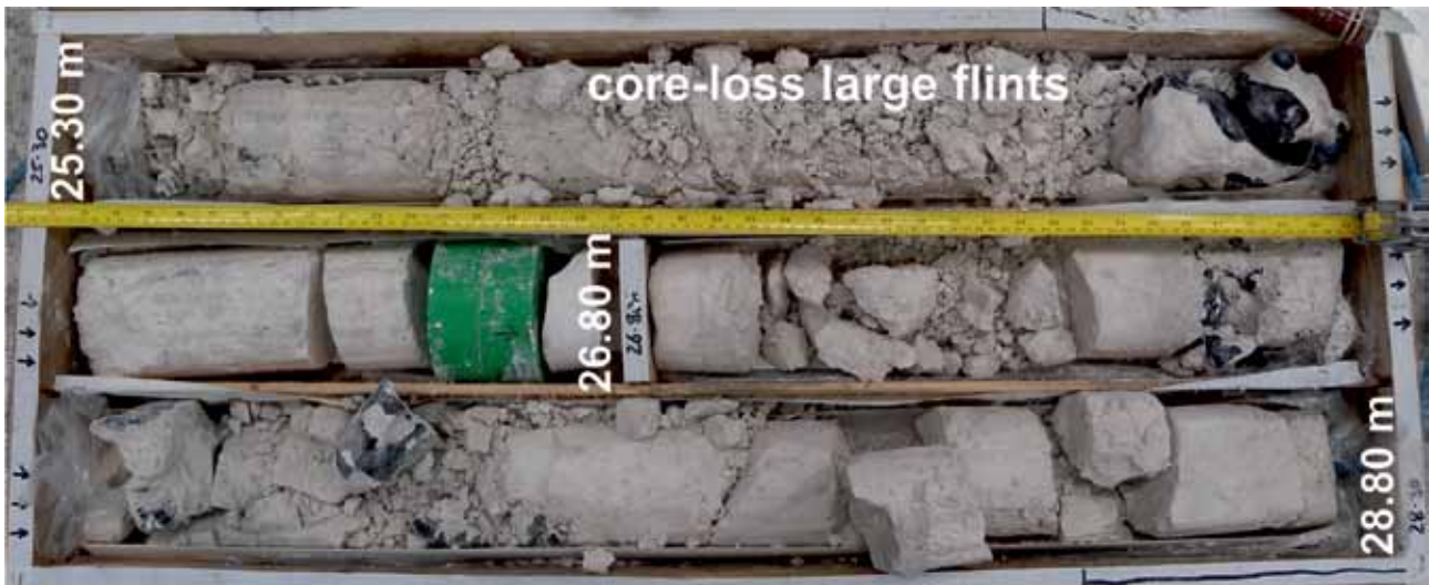
Figure C5c8 Box 7, very large flints in CIRIA grade A chalk. Core fragmentation due to drilling through flints.
