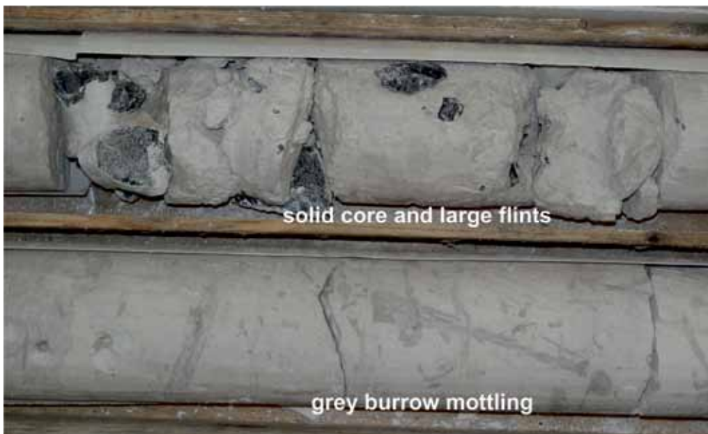
Figure C5a17 Continuously solid core (mostly drilling-induced fractures) with large flints and clean closed joints, CIRIA grade A with abundant light grey trace fossils (burrow-mottled chalk).
