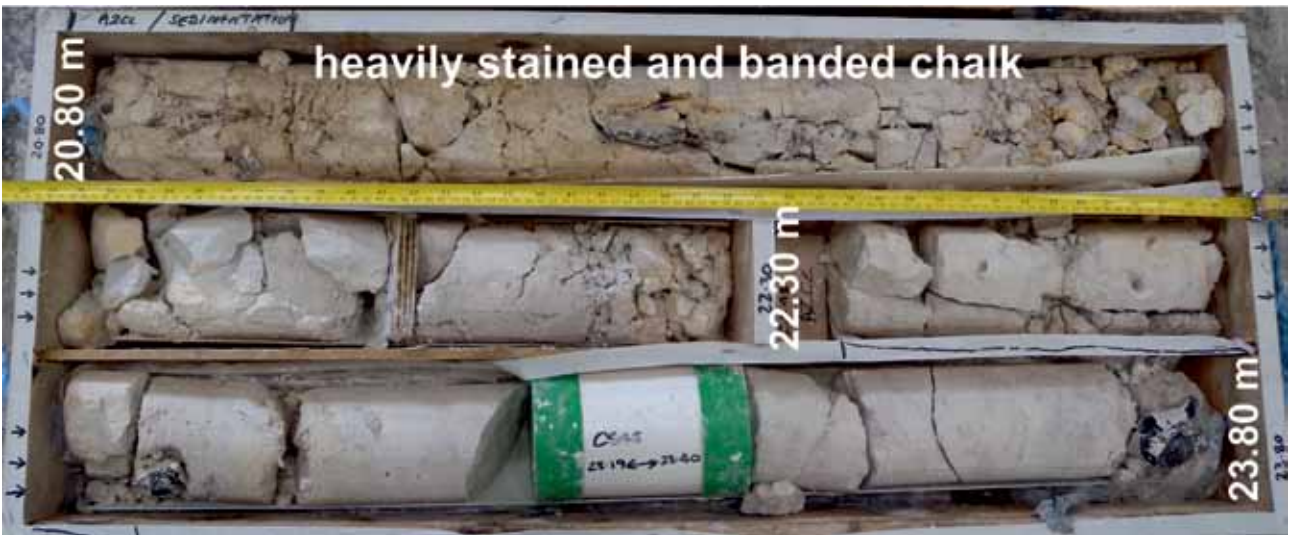
Figure C5c6 One core run with completely fragmented chalk with flints and heavily stained chalk (CIRIA grade B). Below 22.30 m depth the core runs comprise clean chalk with large flints and mostly drilling-induced fractures (CIRIA grade A).
