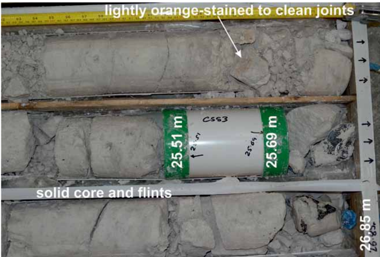
Figure C5a14 Continuously solid core (mostly drilling-induced fractures) with large flints and clean to lightly orange-stained closed joints, CIRIA grade A.
