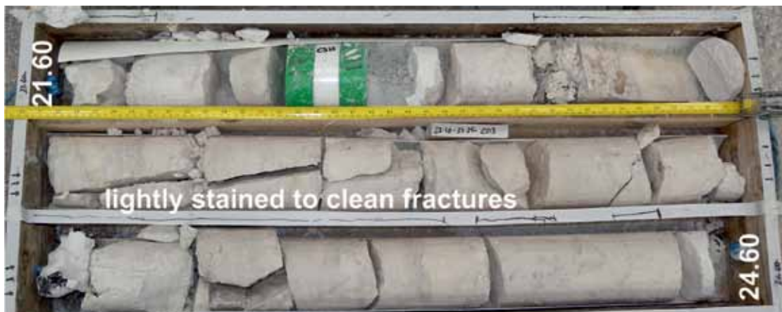
Figure C5b5 WP43R: next box fractures are closed to open <3 mm, clean or lightly stained, hence CIRIA grade A/B.
