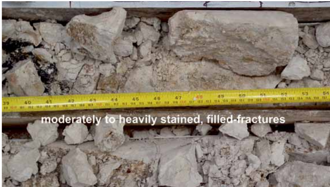
Figure C5b3 Fractures in first 2 m below Thanet contact are open >3 mm, stained and filled, hence CIRIA grade C.
