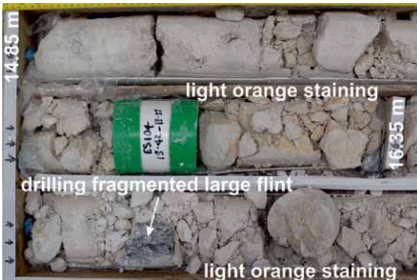
Figure C5a5 Relatively unweathered chalk at the contact between the Chalk and Thanet Sands (CIRIA grade B) and core destructured by drilling. There is light orange staining on joints and internally in the Chalk core.
