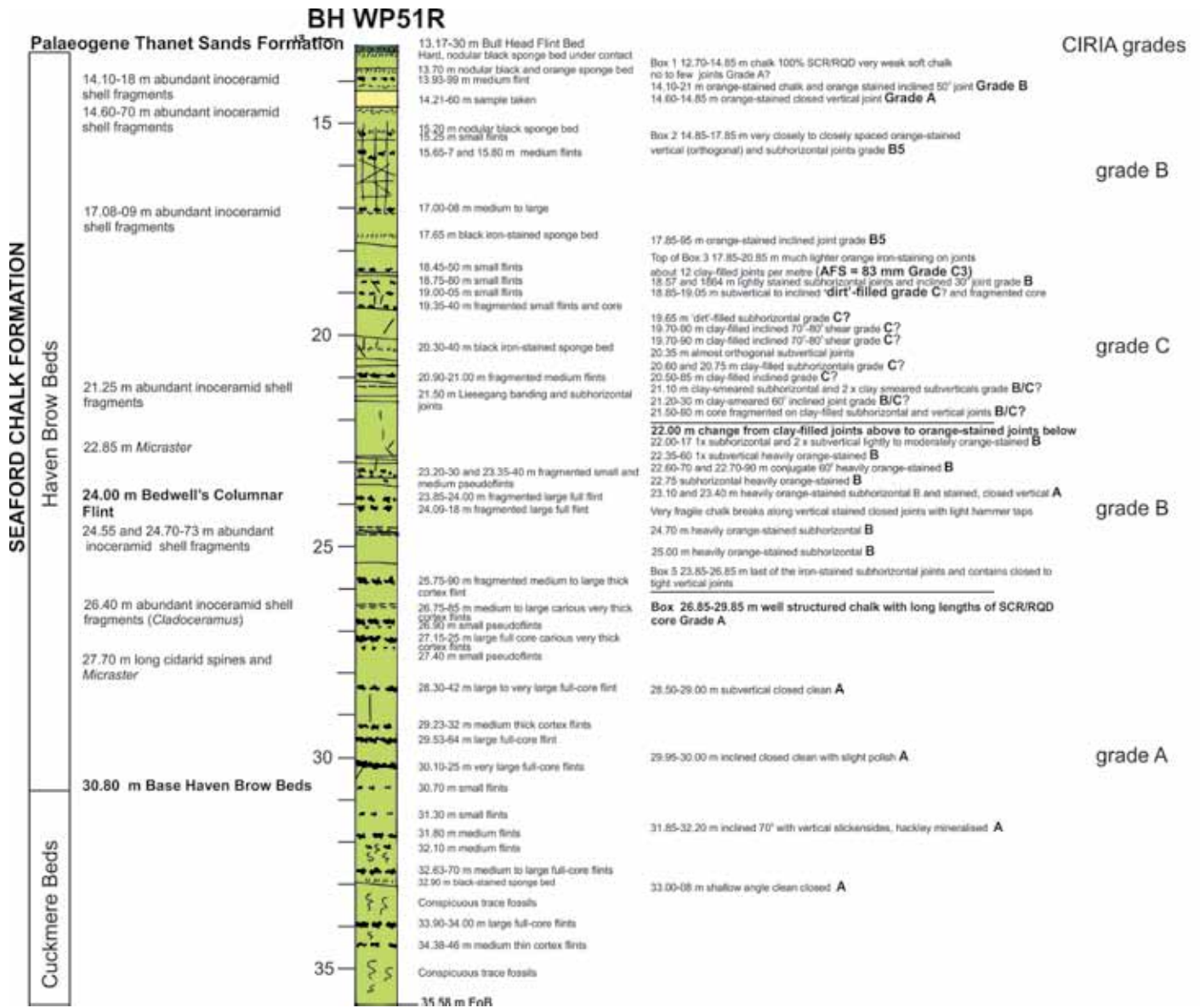
Figure C5a18 Borehole 5a log (East London), illustrating change of CIRIA grade with depth for the borehole cores illustrated in preceding figures.
