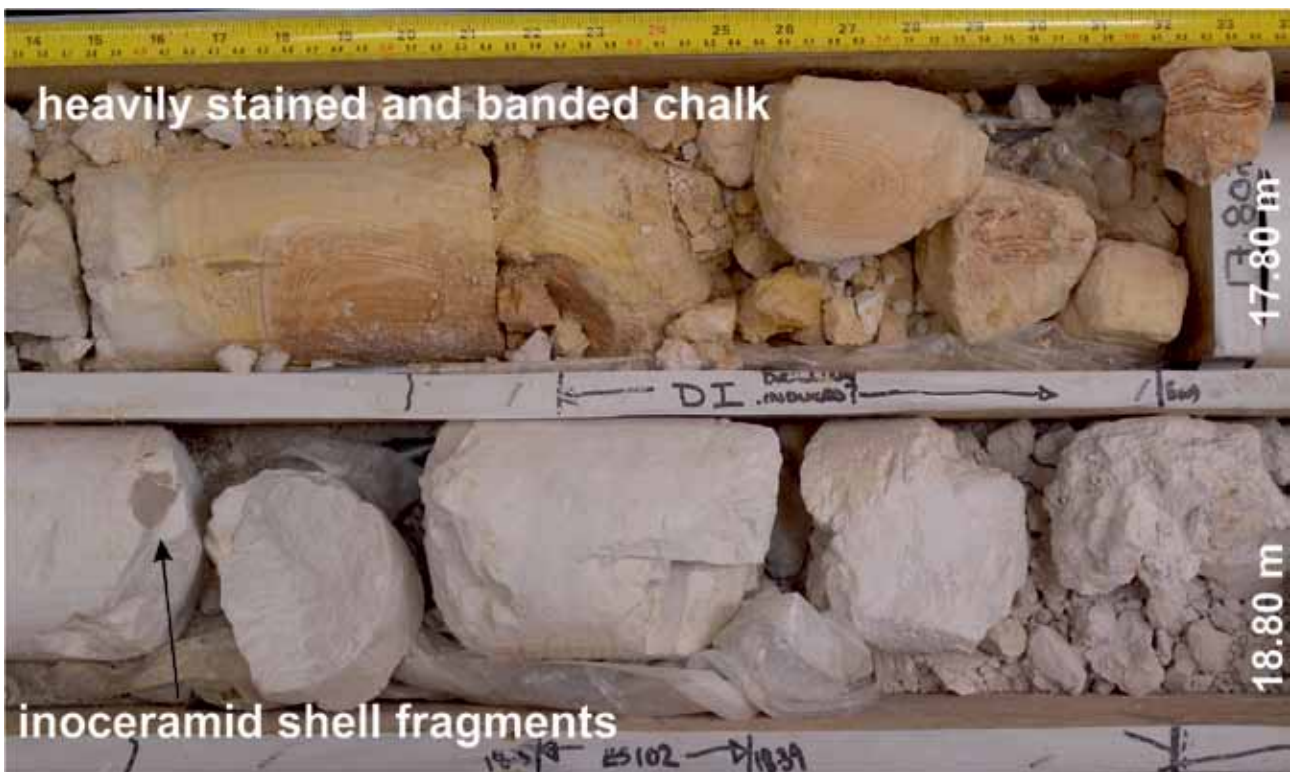
Figure C5c4 Close-up of box 3, heavily stained and banded chalk and vertical joint and some solid core with a closed vertical joint, CIRIA grade B, locally A.
