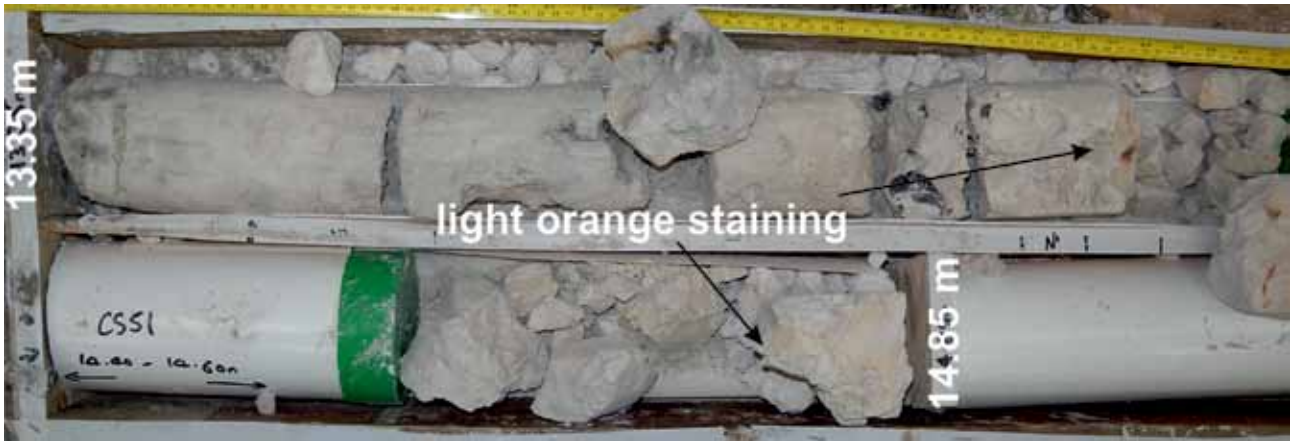
Figure C5a3 Relatively unweathered chalk at the contact between the Chalk and Thanet Sands (CIRIA grade B) and core destructured by drilling. Light orange staining on joints and internally in the Chalk.
